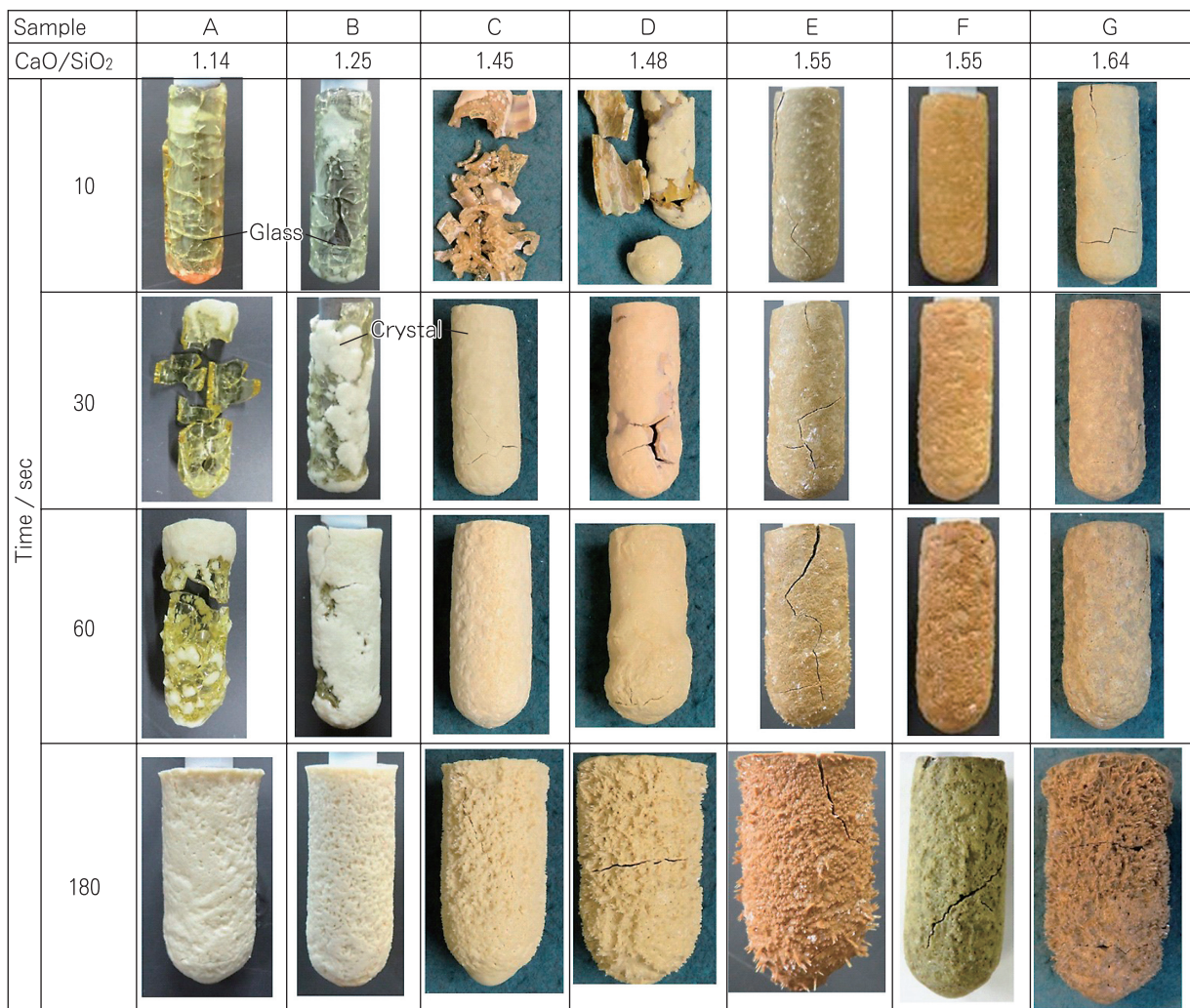
Fig.2 Characteristics of test samples and slag film appearances.
